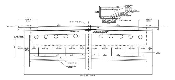
Figure 3 Tunnel Roadway Cross Section
