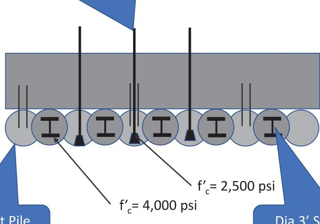
Dia 3' Primary Secant Pile, C-C Spacing = 5.5ft Dia 3' Secondary Secant Pile, C-C Spacing = 5.5ft
