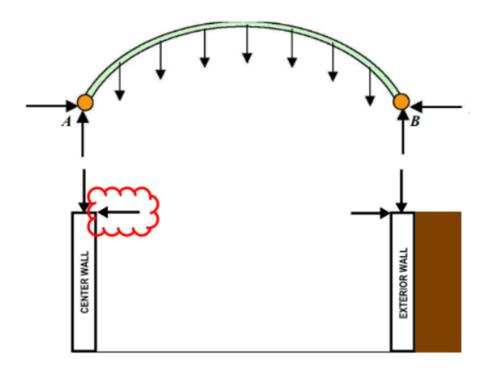
Figure 4 Unbalanced Horizontal Thrust on Center Wall during Construction
