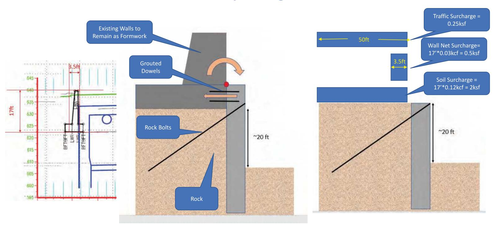
Rock bolt, Drill Hole =0.5ft, At Top, One Row, Incline Angle = 30 deg, C-C Spacing = 5.5ft
